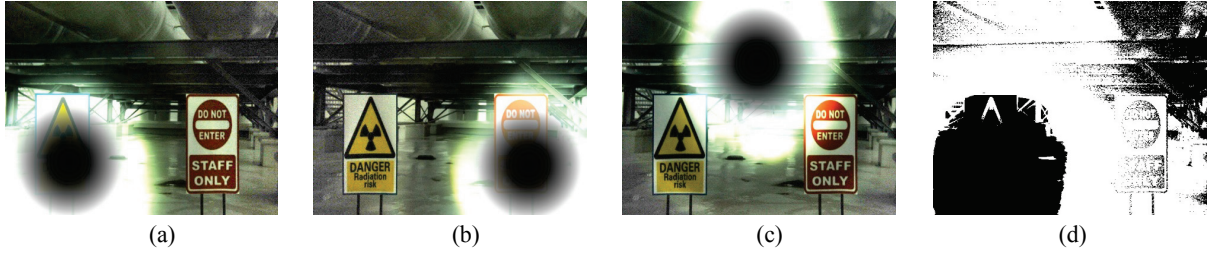
Fig. 5 Luminance corrected images and determination map: (a) Luminance corrected image I_p^1 , (b) Luminance corrected image I_p^2 , (c) Luminance corrected image I_p^3 and (d) determination map D^1 .
