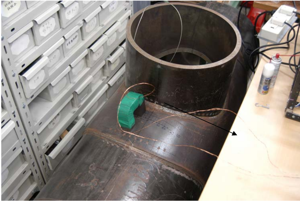
Fig. 3. Photograph of the T-shape tube with the magnetizing yoke placed on the top tube. The arrow shows the direction of movement of the magnetizing yoke ( x direction).
