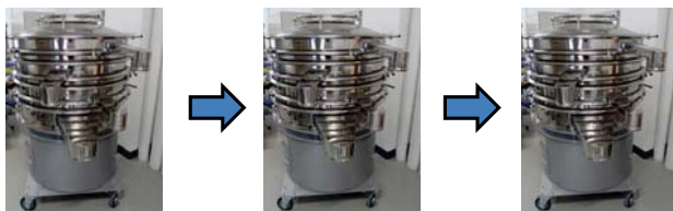
汚染粘土の破碎と分級による減容化 (Reduction of volume by fragmentation and classification of contaminated clay)
