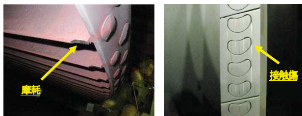
Fig.2 Damage of the turbine blade
